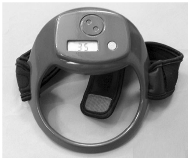
Fig. 1 The non-thermal pulsed radio frequency PEMF device used in this randomized, double-blind clinical study on knee OA pain. The device consists of a single loop wire coil with integrated amplifier (Palermo, Ivivi Health Sciences, San Francisco, CA) that delivers a PRF signal configured to modulate the CaM/NO/cGMP signaling pathway, which consisted of a 7-ms burst of a 6.8 MHz sinusoidal carrier repeating at 2 bursts/s, delivering a peak induced electric field amplitude of 34 \pm 8 V/m in the knee. The device is portable and easily positioned by the patient over the knee with the Velcro™ strap. The number displayed is the number of PEMF treatments
